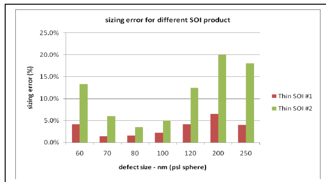
Figure 3. Defect sizing error for different substrate products, demonstrating the necessity for specific calibration curves.
