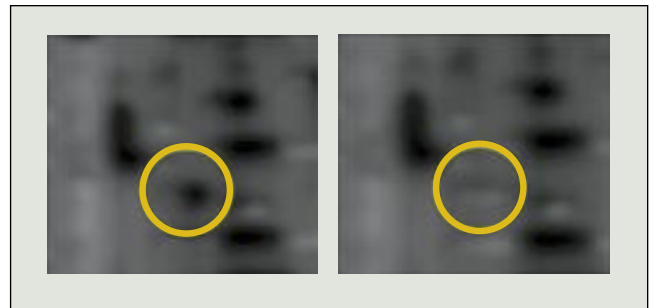
Figure 4. Material contrast seen through an etched local interconnect level prior to \bar{W} fill.
