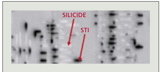
Figure 3. Material contrast seen through an etched local interconnect level prior to \bar{W} fill.
