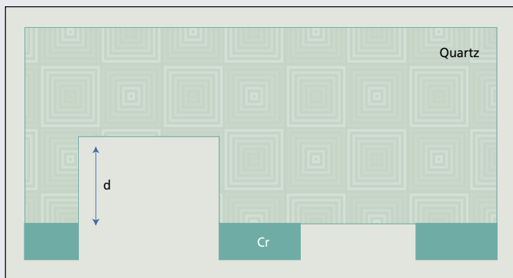
Figure 1. Example of a simple alternating phase shift mask manufacturing approach.
