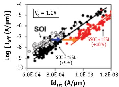
Figure 8:  $I_{d,sat} - I_{off}$  plot showing the nFET enhancement due to tESL & SSOI.
