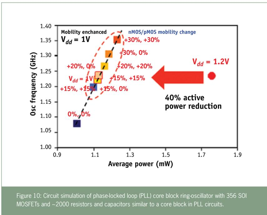
Figure 10: Circuit simulation of phase-locked loop (PLL) core block ring-oscillator with 356 SOI MOSFETs and ~2000 resistors and capacitors similar to a core block in PLL circuits.
