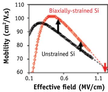
Figure 6: Long-channel hole mobility showing the strong sensitivity of the biaxially strained Si enhancement as a function of effective vertical field.
