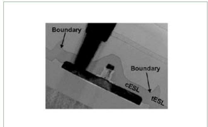
Figure 1: High resolution TEM of an isolated poly pitch, small SA pMOS device in a "compressive-first" dESL stressor.
