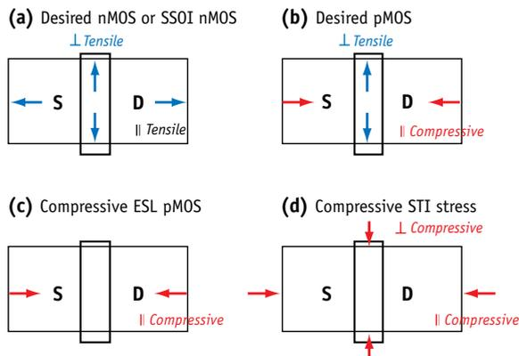
Figure 7: Schematic showing various stress configuration and their associated stressors.
