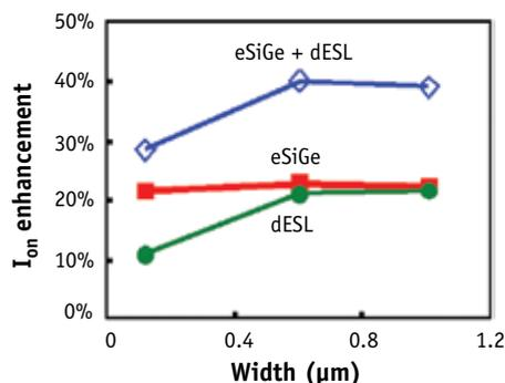
Figure 5:  $I_{on}$  enhancement as a function of device width for different strained devices.
