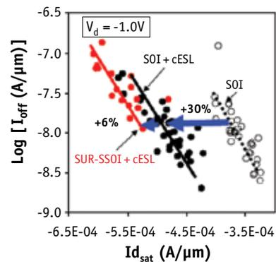
Figure 9: Short-channel pFET  $I_{d,sat} - I_{off}$  plot showing the enhancement due to SUR and cESL ( $W = 1\mu m$ ).
