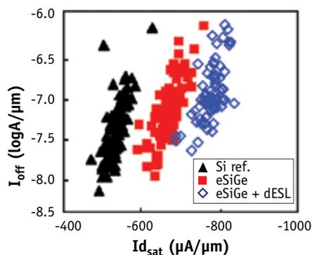
Figure 4: Off current as a function of drive current for strained and unstrained pMOS devices.
