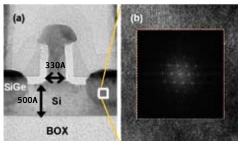
Figure 3: 65nm strained pMOS: a) device structure; b) HR-TEM and Fourier transform diffractogram from S/D SiGe region for crystallinity characterization.
