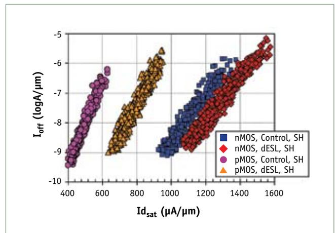
Figure 2: 1.2V pMOS and nMOS self-heated (SH)  $I_{off} - I_{dsat}$  curves for dESL integration with -650MPa compressive and +400MPa tensile lateral channel stresses.
