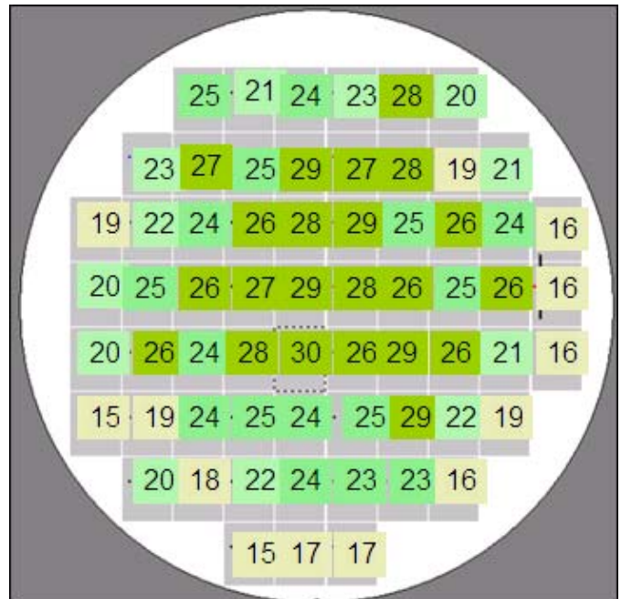
Figure 7: Gate line width delta (dLWp) from the VC test structure
