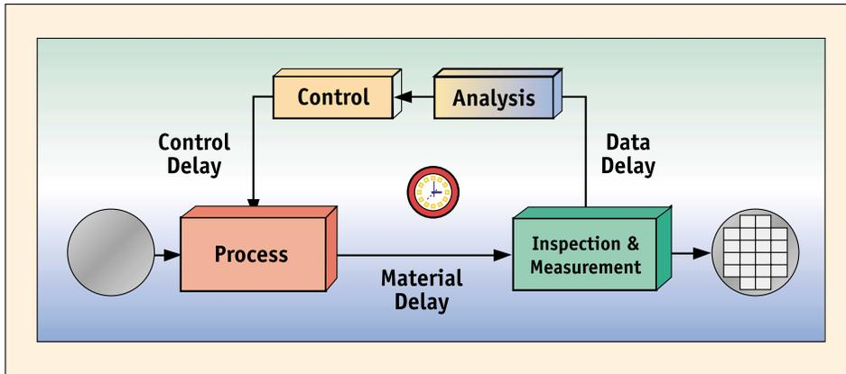
Figure 8. Flow for a process step.
