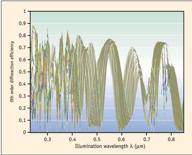
Figure 6. Reflectance, R, as a function of the illuminating wavelength, λ.
