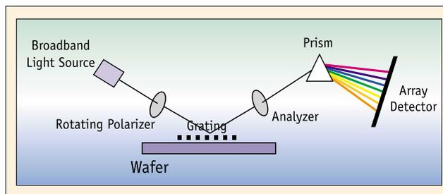
Figure 1. Schematic of SCD measurement on a KLA-Tencor SpectraCD.
