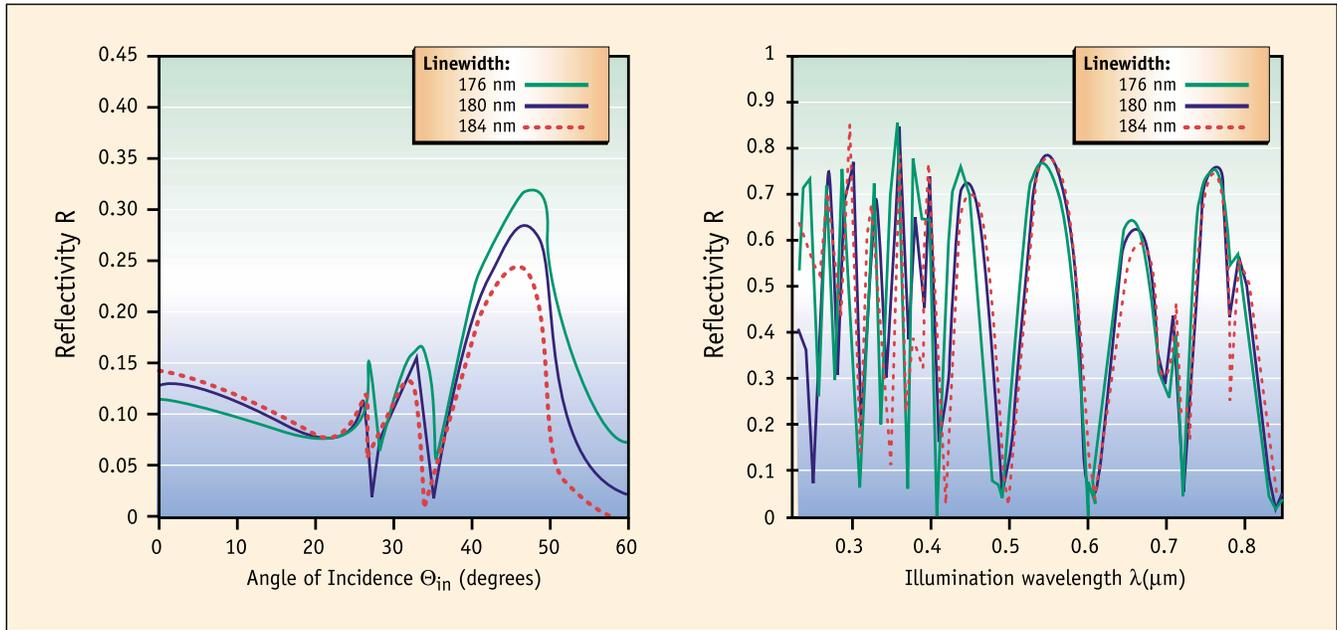
Figure 4. Reflectance,  $R$ , versus angle of incidence,  $\theta_{in}$ , and illumination wavelength,  $\lambda$  ( $\mu\text{m}$ ), from simulation as in Figure 2 with lines for  $0.18 \mu\text{m} \pm 4 \text{ nm}$  added.
