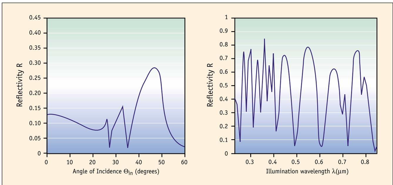
Figure 3. Reflectance, R, versus angle of incidence,  $\theta_{in}$ , and illumination wavelength,  $\lambda$  ( $\mu\text{m}$ ), from simulation of 0.18  $\mu\text{m}$  resist lines in a 50% duty cycle grating (1  $\mu\text{m}$  resist thickness, square profile, bare silicon substrate).
