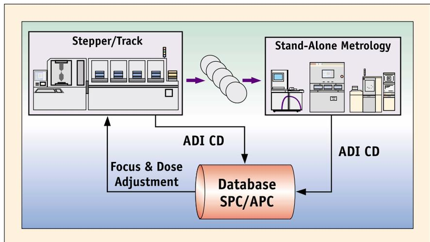
Figure 9. SCD integrated onto a stepper/track module.
