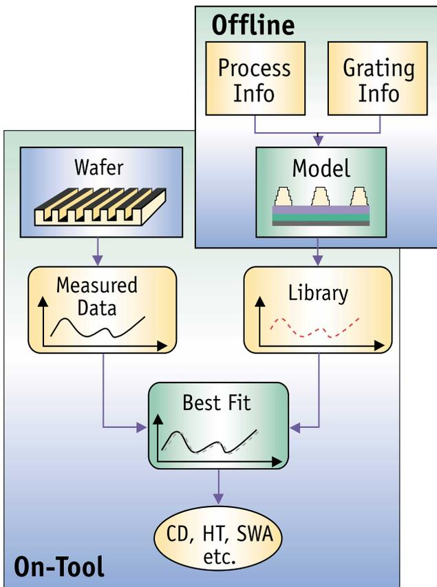
Figure 2. SCD measurement flowchart.
