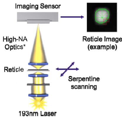
Figure 5: Mask inspection tool image acquisition (transmitted light case shown)
