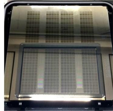
Figure 4: Actual EUV test mask with EUV pellicle covering lower half
