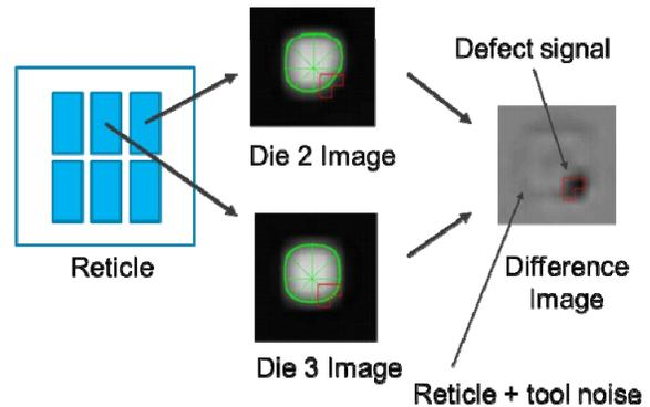
Figure 6: Mask inspection tool image processing (optical mask case shown)
