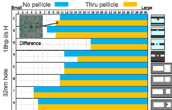
Figure 12: Inspection comparison without pellicle vs. with pellicle showing defects detected
