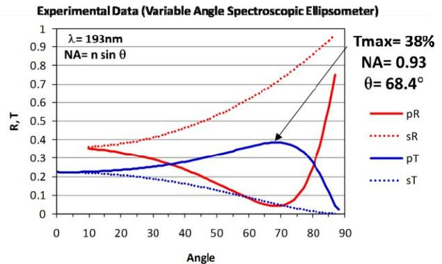
Figure 2: Pellicle transmission and reflection at  $\lambda = 193\text{nm}$
