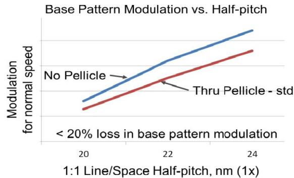
Figure 8: Base pattern modulation comparison without pellicle vs. with pellicle for different line/space half-pitches
