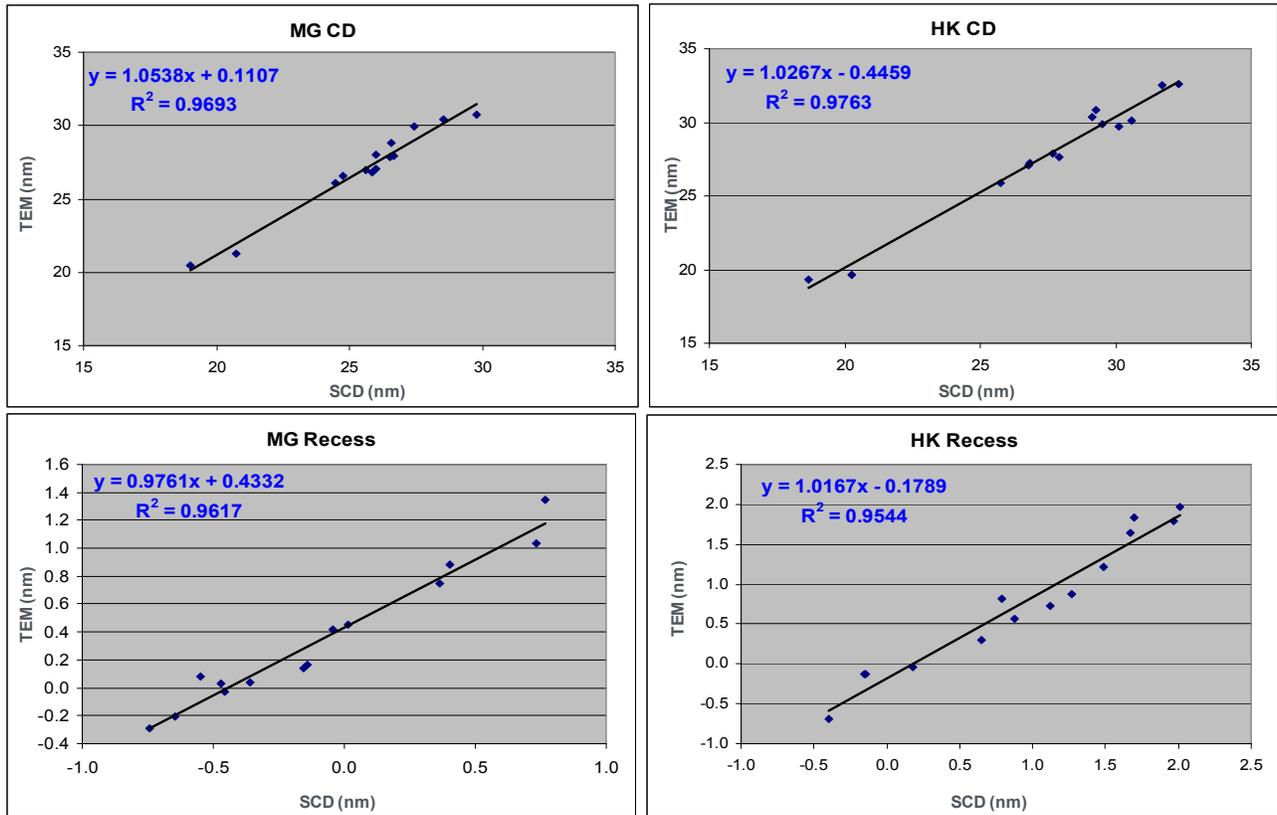
Figure 10. MG/HK CD and MG/HK recess correlation between SCD tool and TEM reference.
