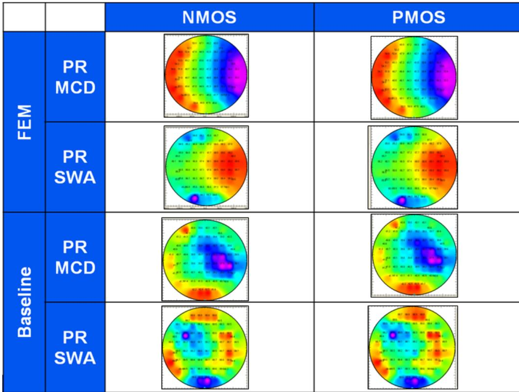
Figure 4. Wafer maps of MCD and SWA for DOE wafer and baseline wafer.
