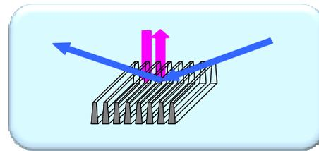
Figure 1b. Schematic of multi-channel scatterometry.
