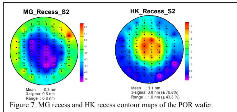
Figure 7. MG recess and HK recess contour maps of the POR wafer.
