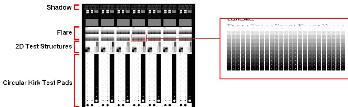
Figure 1: The EUV test reticle is composed of seven identical, vertical layouts. Within each layout is a shadowing test structure, a flare test structure, a set of 2D test patterns (such as line-end shortening), and a flare Kirk test pattern. The pattern density for the full field is shown on the left, and on the right is a detail of the flare pattern density test structure.
